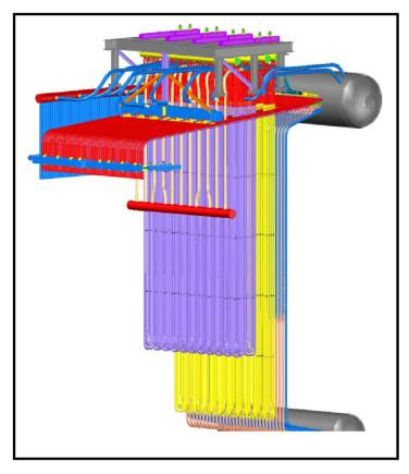
The project work included defining target process conditions, deriving conceptual design options, sizing the new superheaters, material selection, preparing equipment specifications, and supplying the fabrication and installation drawings.
