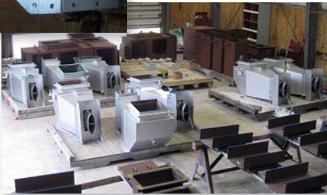
Components of OFA Upgrade on Boiler "B" in the Fabrication Shop
